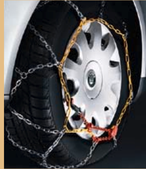
Snow chains for 15" wheels and tyres 195/65 R15 (CEP 300 002A) Snow chains for 16" wheels and tyres 205/55 R16 (CEP 300 003)
