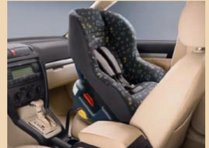
Child seat Bimbo Fix (DDF 000 001 for rear-facing fittings, DDF 000 004 for forward-facing fittings) Bimbo Fix child seat frame fittings (DDF 000 003 for rear-facing fittings, DDF 000 002 for forward-facing fittings)
