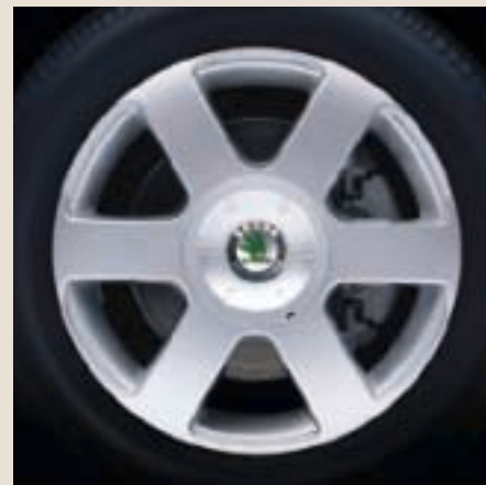
Alloy wheel 6,5J x 16" Vega for tyre 205/55 R16 (CCR 600 005)
